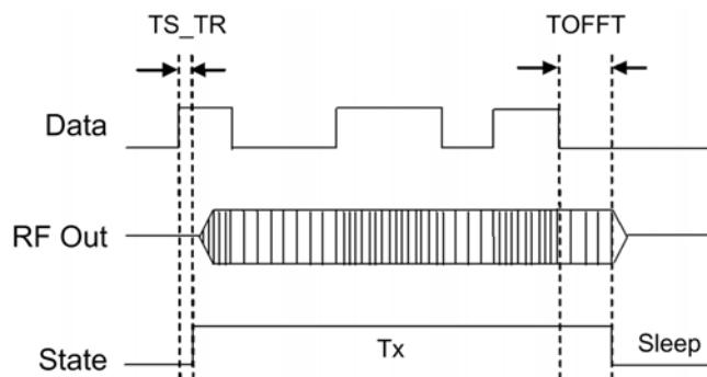
Figure 3. ‘Power & Go’ Mode: Transmitter Timing Operation
