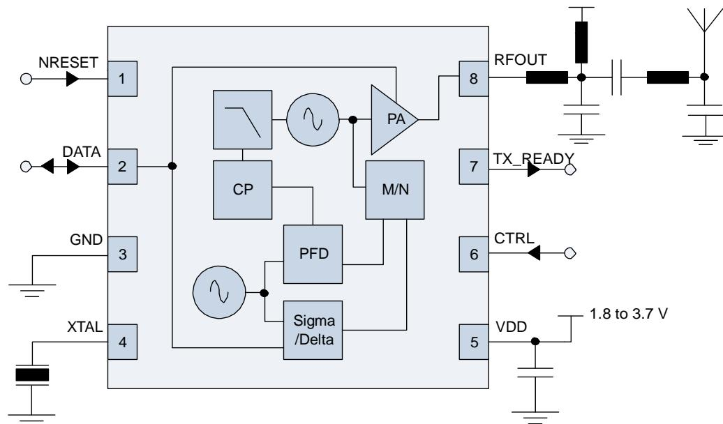
Figure 1. HC1243 Simplified Block Diagram
