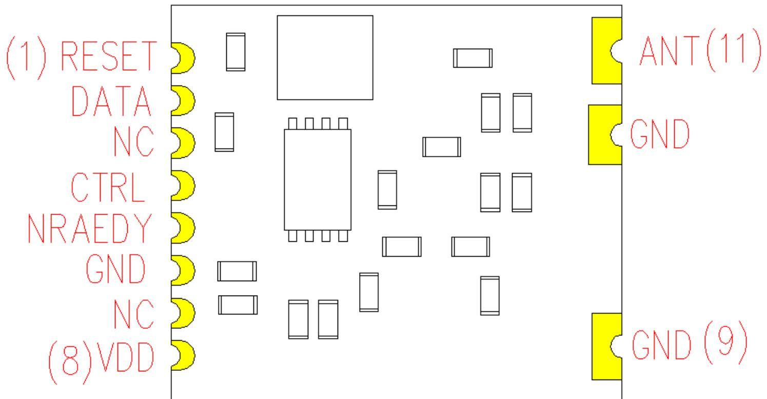
Figure 2. Pin Configuration
