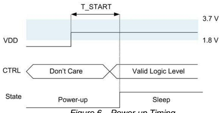
Figure 6. Power-up Timing
